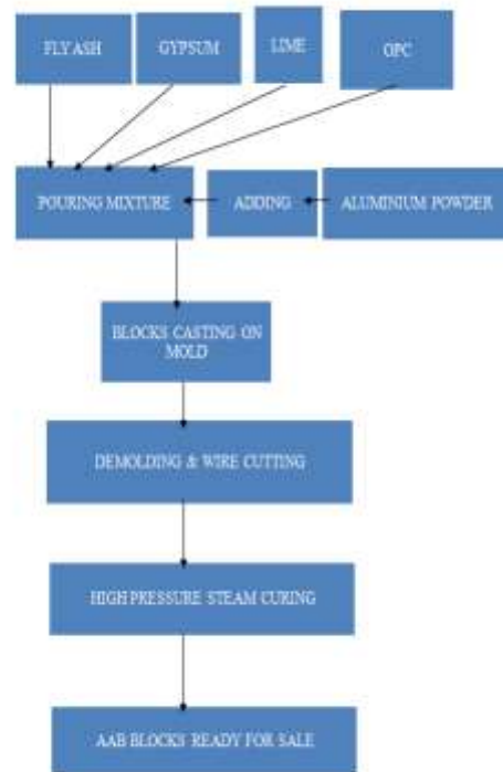
Fig 1.1: Flow chat of AAC Blocks Preparation Method
