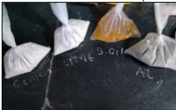
Fig 6.1: Binder Material Used In AAC Manufacturing
