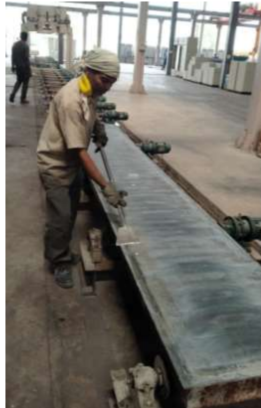
Fig 6.7: Mould Plate Cleaning Before implementing MPCM Process
