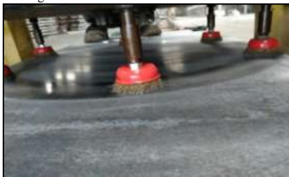
Fig 6.6: Mold Plate Cleaning Process (Close Up)
